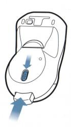
15 Insert the USB Receiver into the USB storage compartment. Push gently until it clicks in place. Push gently again to release.
